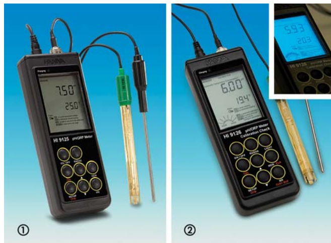
Portable pH-/mV-/°C-meters HI 9125 and HI 9126 By Hanna.
